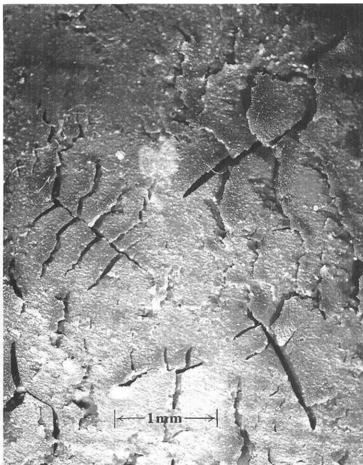
Figure 9. A close-up view of cavitation cracks in a lightly carbon black filled vulcanisate (Compound 1). At a stress approaching break, secondary cracks can propagate from the primary cracks normally at an angle of approximately 90^\circ .
