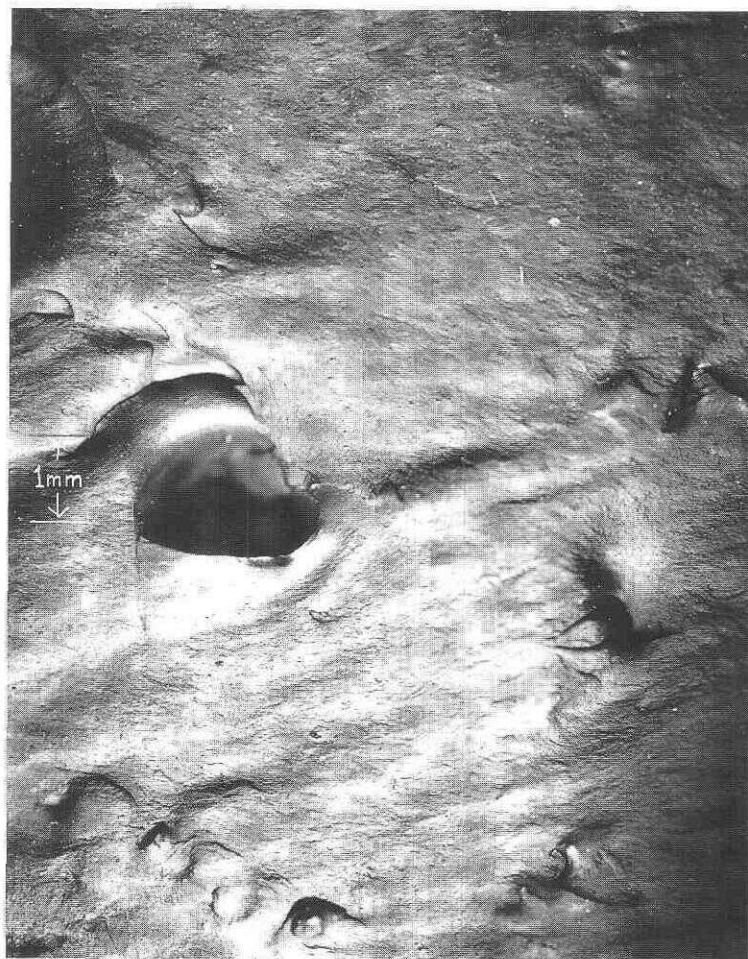
Figure 10. A typical crack face and cavity in a highly carbon black filled vulcanisate (Compound 5) pulled to break. The crack face is relatively featureless when compared to an intermediate filled vulcanisate.
