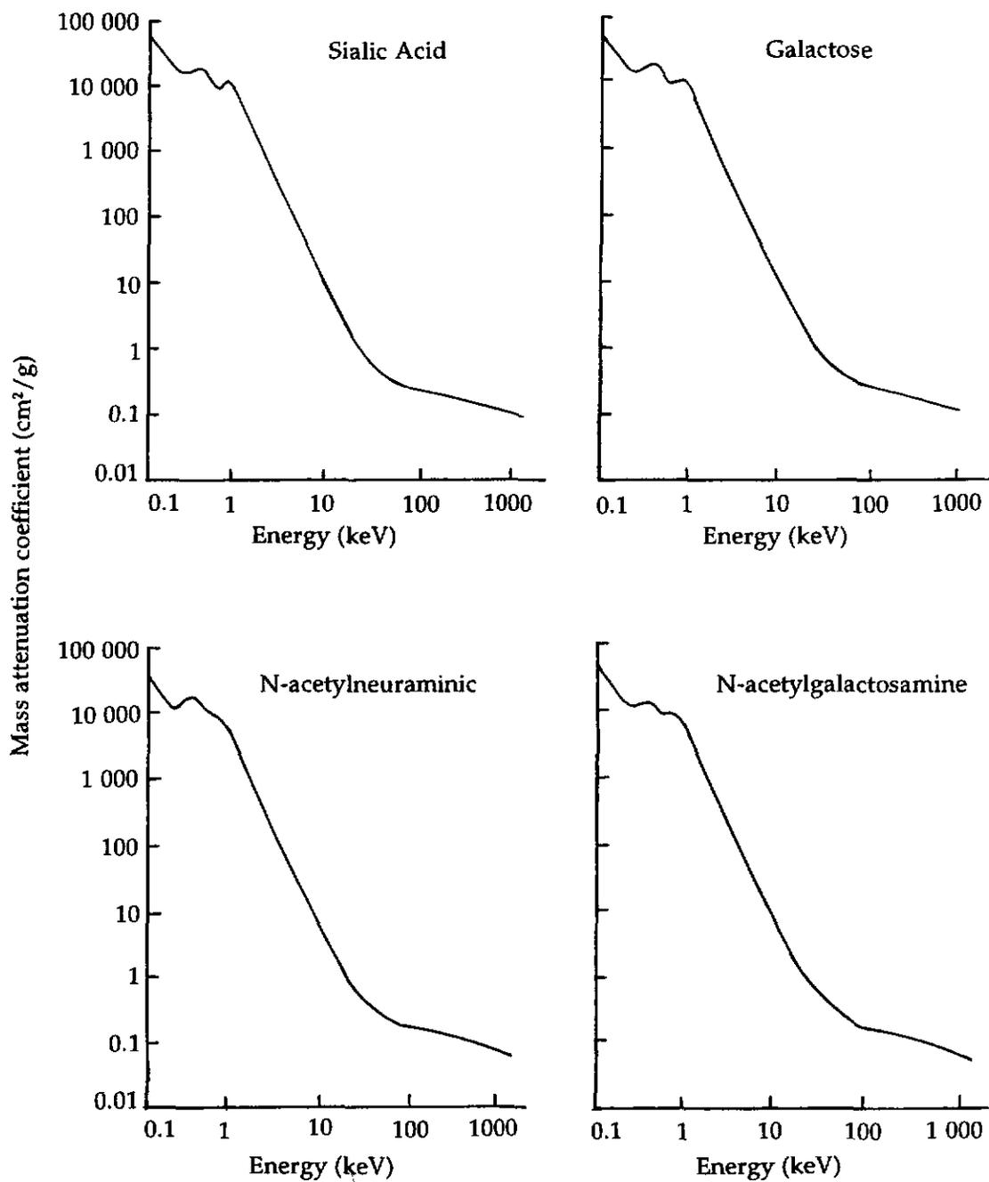
Figure 2. Mass attenuation coefficients of some non-rubber constituents of natural rubber.
