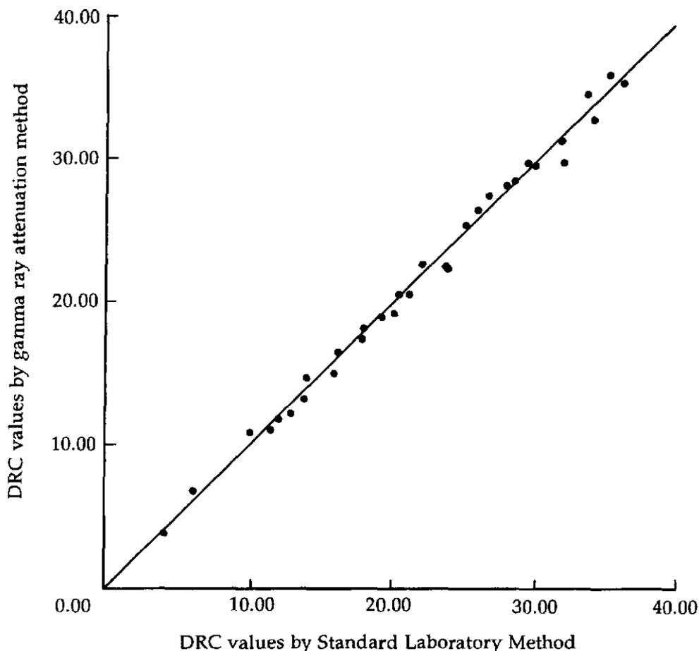
Figure 4. Typical relationship between dry rubber content measured by the  $\gamma$ -ray attenuation method and standard laboratory method.
