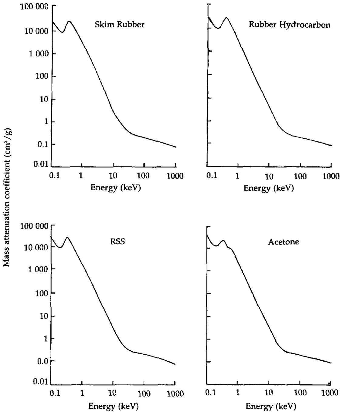
Figure 1. Mass attenuation coefficients of skim rubber, RSS, rubber hydrocarbon and acetone extract.
