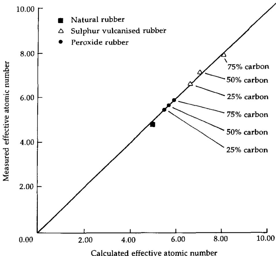
Figure 3. Correlation between calculated and measured effective atomic number of natural rubber, and sulphur and peroxide vulcanised rubbers.
