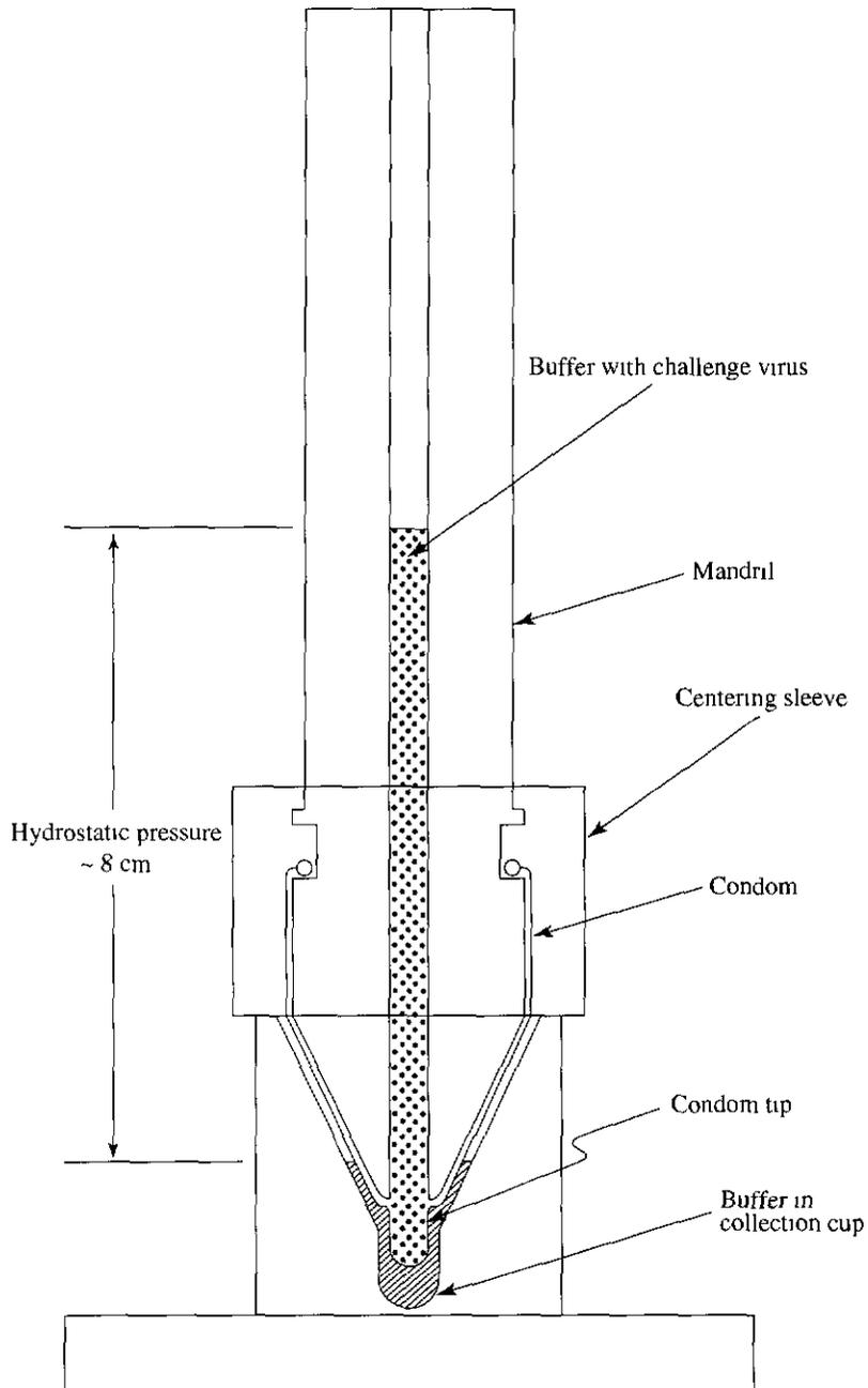
*Figure 1 Schematic diagram of low-pressure condom test apparatus
