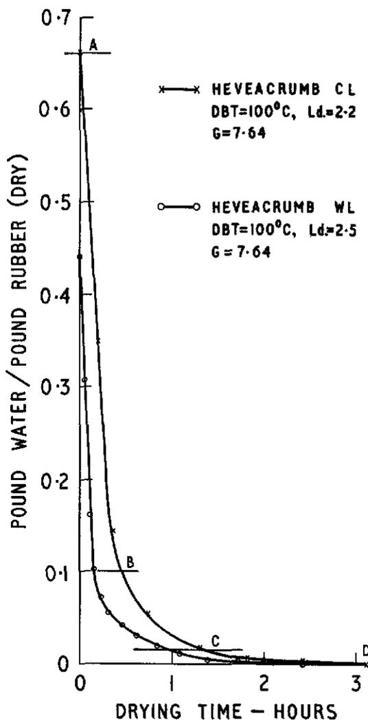
Figure 2. Typical drying curves for Heveacrumb WL and CL.
