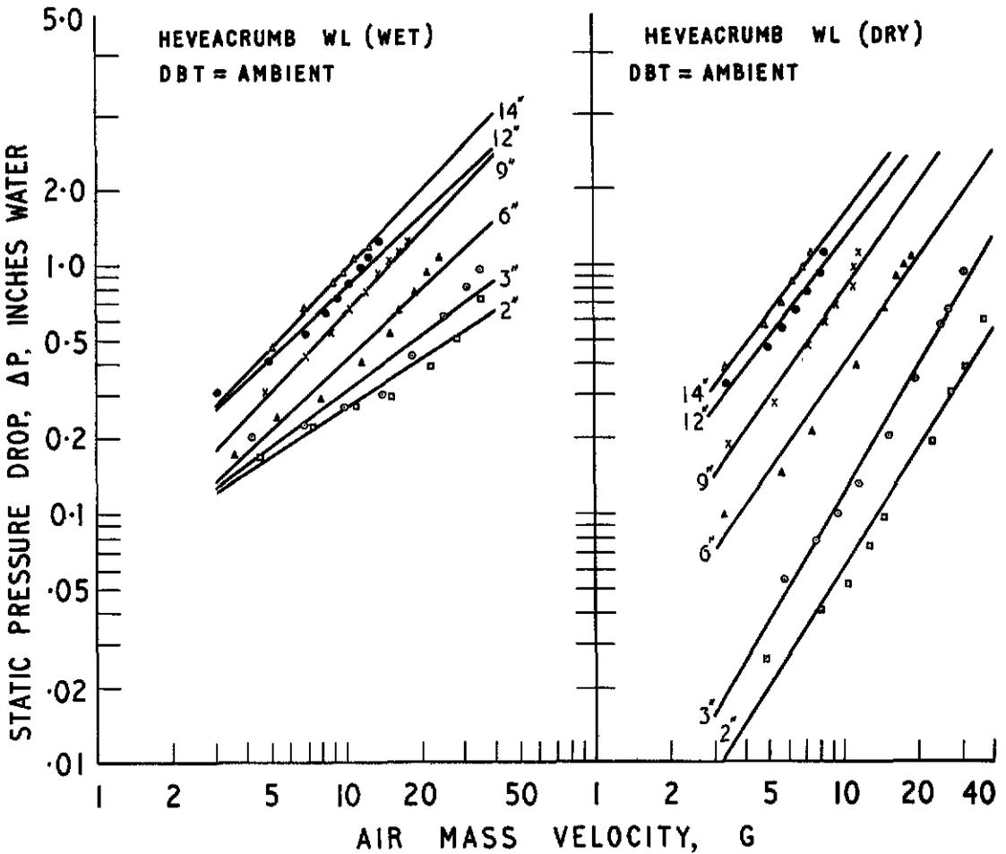
Figure 8. Variation of static pressure drop with air mass velocity and loading depth.
