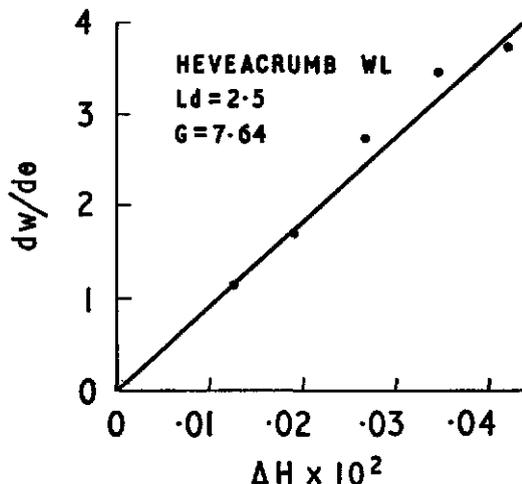
Figure 4. Effect of temperature and humidity on the drying of Heveacrumb WL during the constant rate period.
