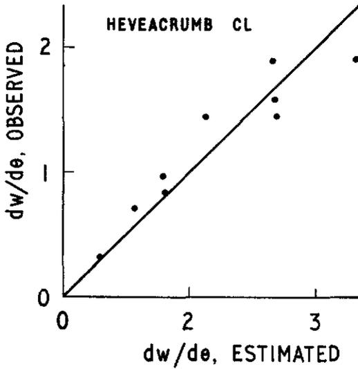
Figure 10. Verification of observed and estimated rate of drying during constant rate period—Heveacrumb CL.
