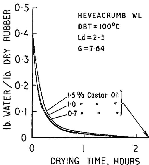
Figure 13. Drying curves for Heveacrumb WL with various concentrations of castor oil.
