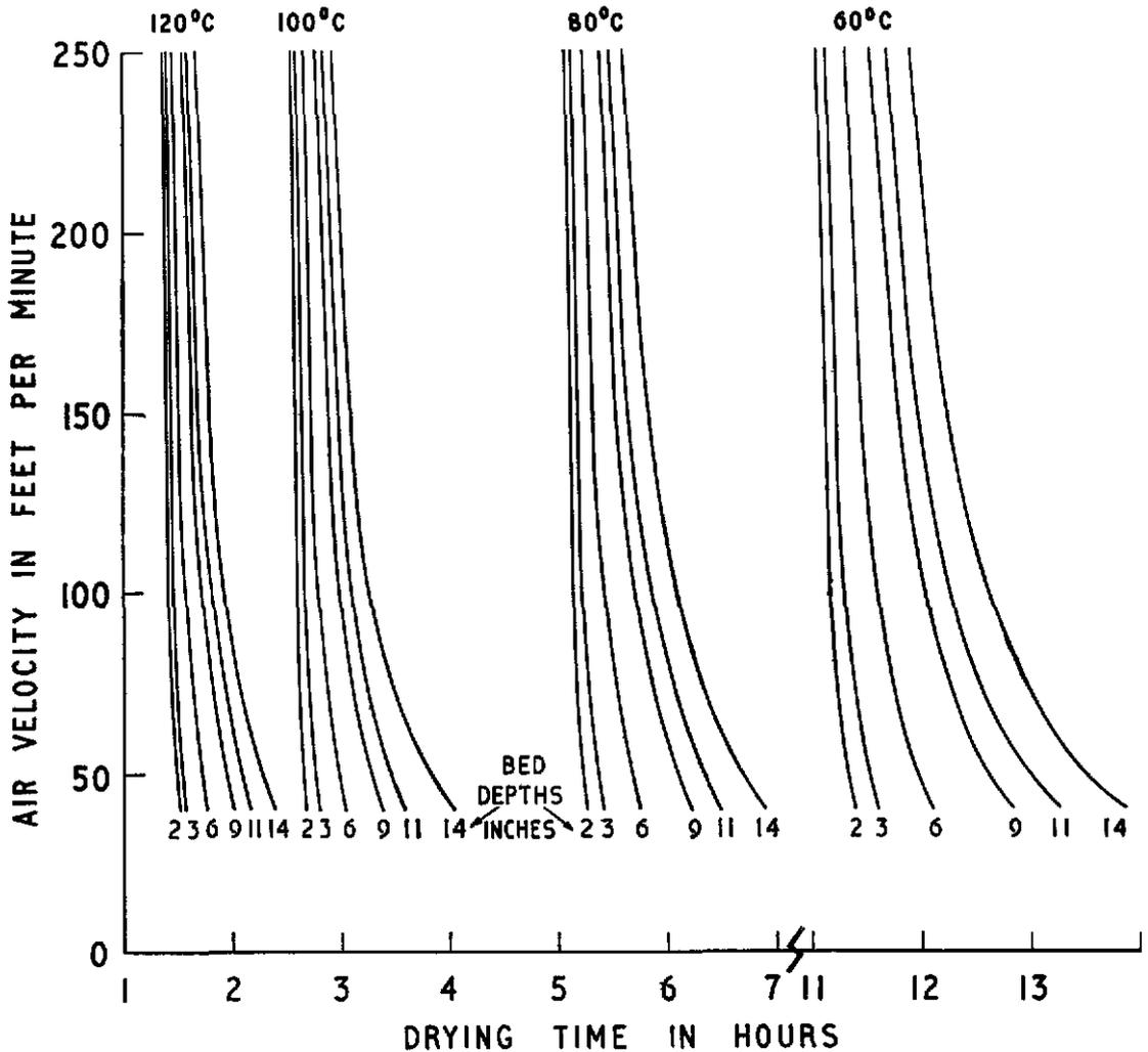
Figure 12. Summary of the effect of temperature, the loading rate and the air velocity on total drying time of Heveacrumb WL.
