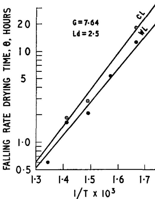
Figure 11. Correlation of drying temperature with falling rate drying time.
