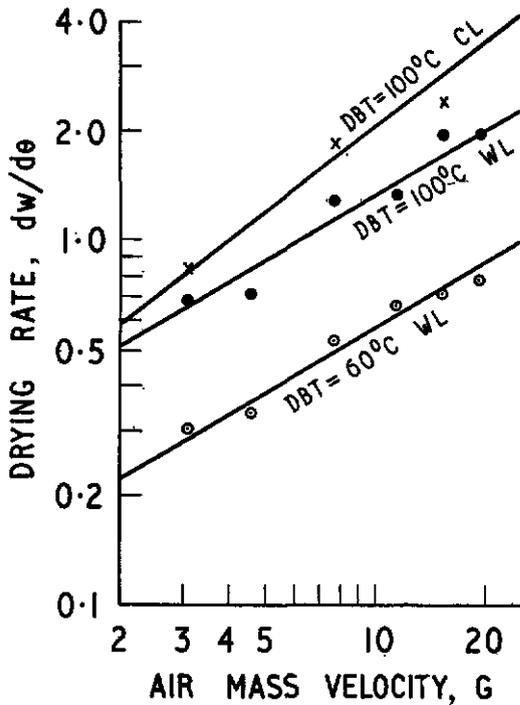
Figure 5. Effect of air mass velocity on drying of Heveacrubm WL and CL during the constant rate period. ( $L_d = 2.5$ ).
