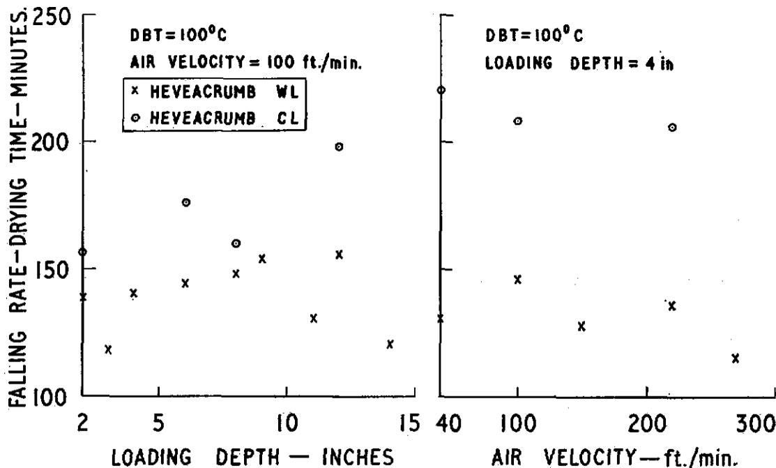
Figure 7. Effect of loading depth and air velocity on the falling rate drying time.
