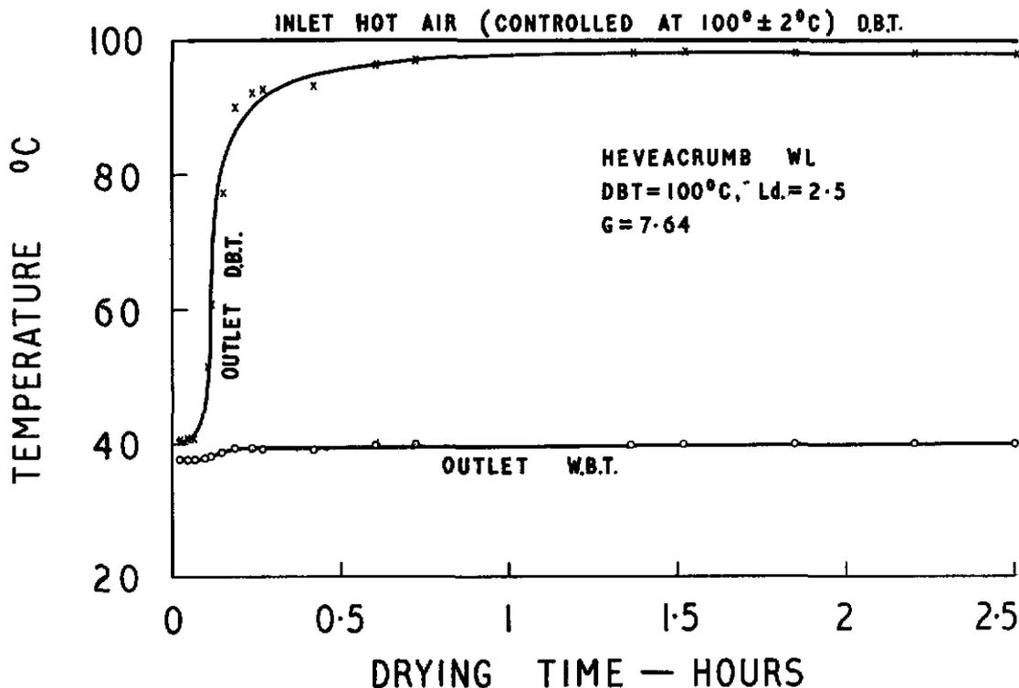
Figure 3. Typical variation of dry and wet bulb temperatures while drying Heveacrumb WL.
