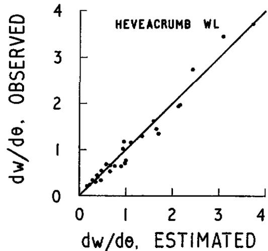
Figure 9. Verification of actual (observed) and estimated rate of drying during constant rate period—Heveacrumb WL.
