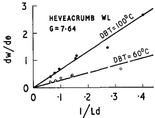
Figure 6. Effect of loading rate on drying of Heveacrubm WL during the constant rate period.
