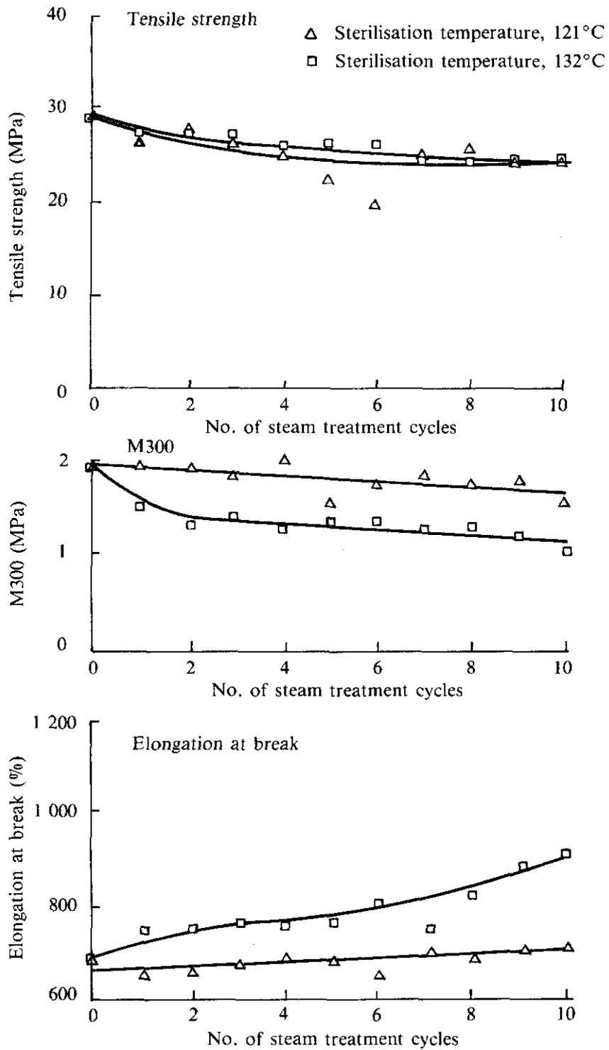
Figure 3. Effect of steam sterilisation on tensile strength, M300 and elongation at break for Cure System B.
