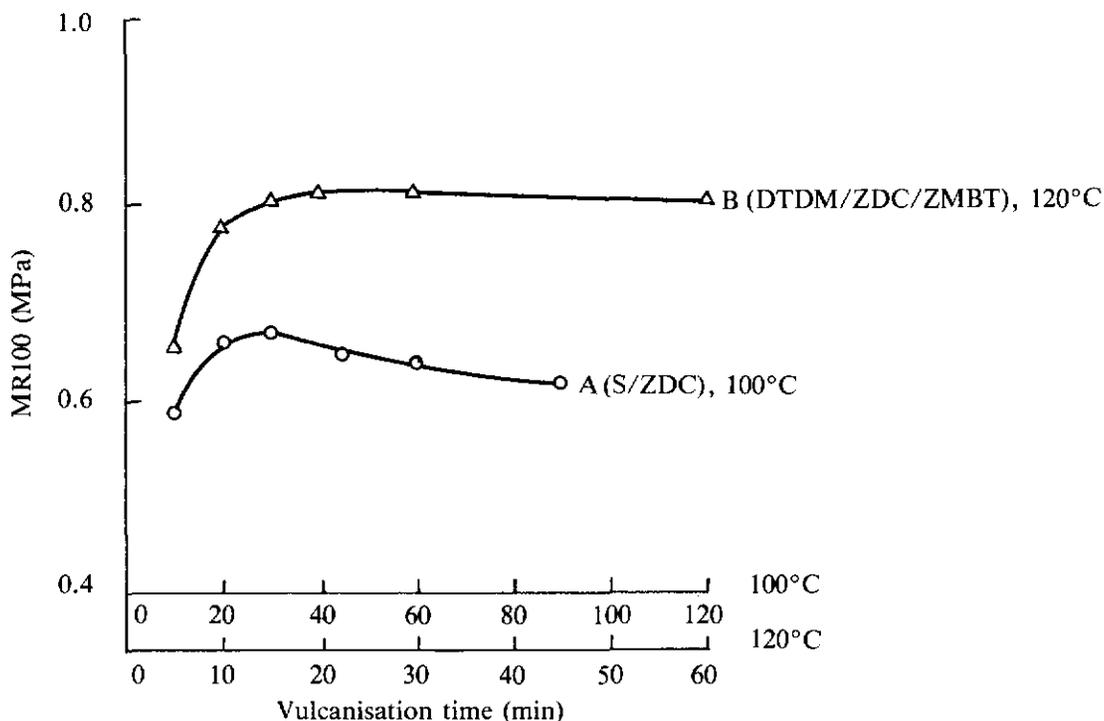
Figure 1. Vulcanisation kinetics of latex films of conventional high sulphur (S/ZDC) and sulphur-donor (DTDM/ZDC/ZMBT) cure systems.
