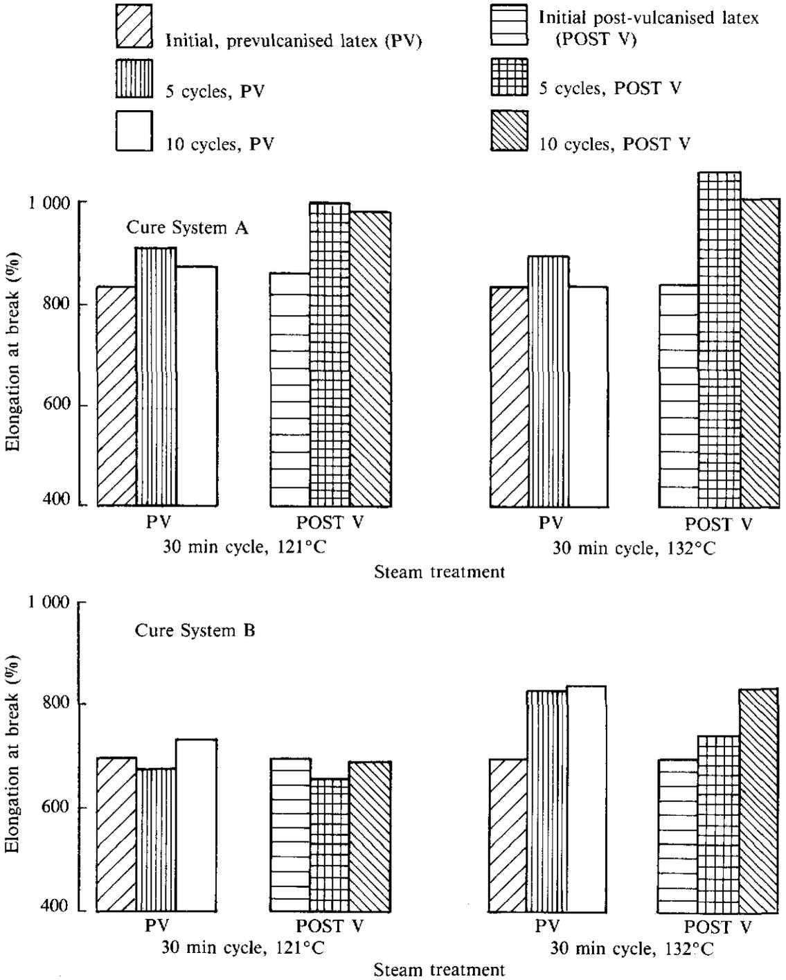
Figure 8. Elongation at break of prevulcanised and post-vulcanised latex films after steam treatment for Cure System A and Cure System B.
