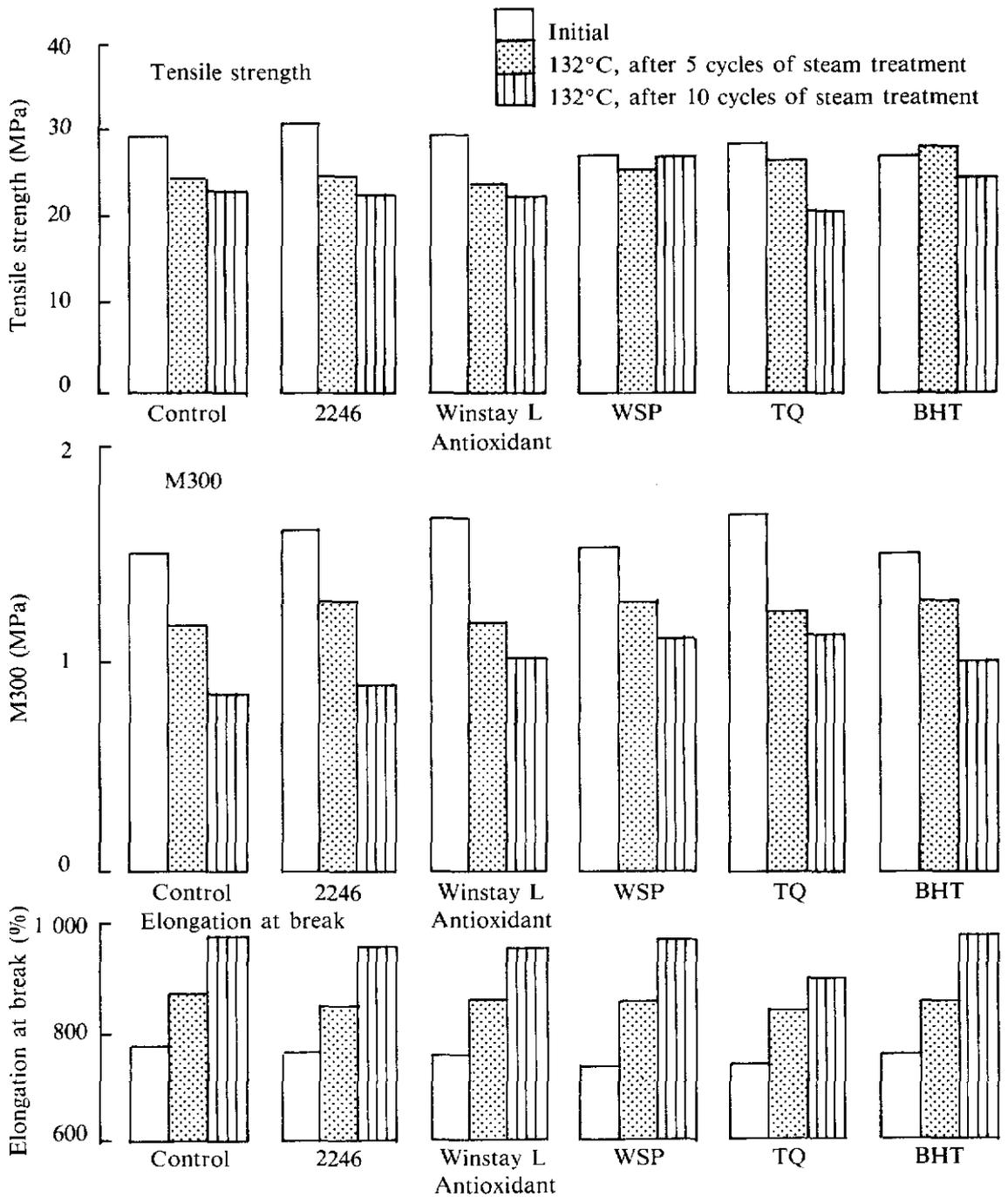
Figure 5. Variation of tensile strength, M300 and elongation at break with antioxidant type after steam treatment for Cure System B.
