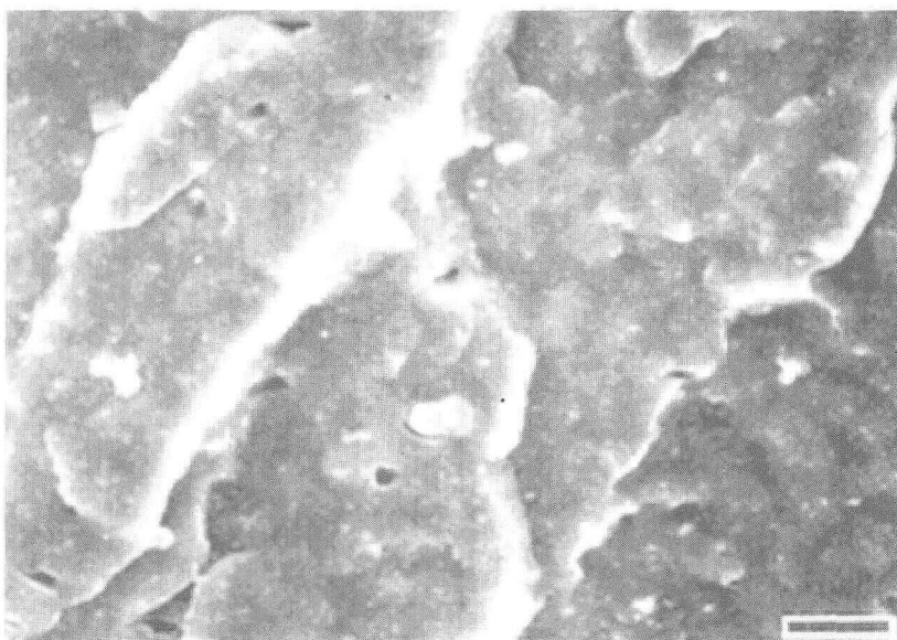
Figure 2. SEM ultra-micrograph of masterbatch from unmodified clay after aging. (Bar = 10 \mu\text{m} .)
