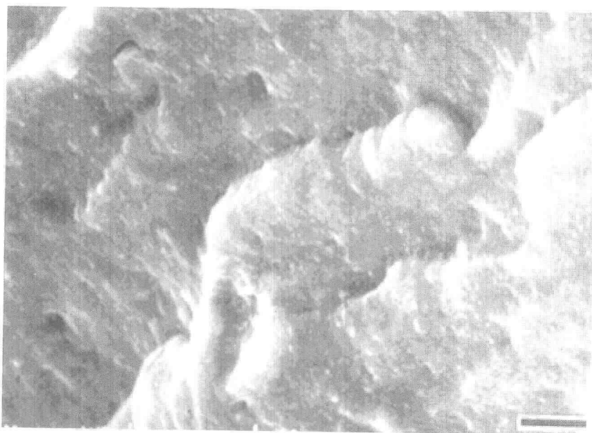
Figure 3. SEM ultra-micrograph of aged Masterbatch F. (Bar = 5 \mu\text{m} .)
