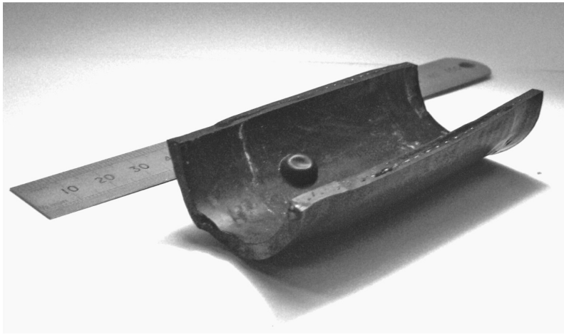
Figure 4. Showing a section of rubber hose after exposure to ECD. A “blister” has formed on the inner wall due to the ingress of liquid coolant into the rubber as a result of ECD.
