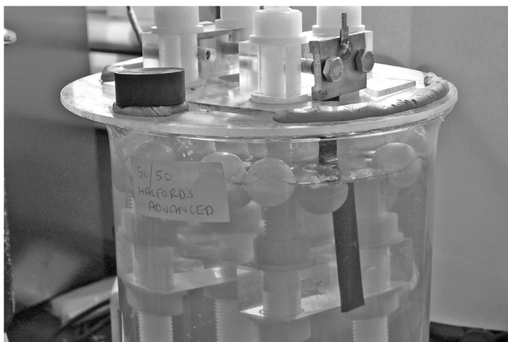
Figure 1. A typical ECD beaker cell test apparatus partially filled with a coolant with a rubber test strip shown in the foreground attached to a fixing clamp for electrical connection.
