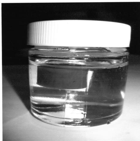
*Figure 1. Showing a sample of rubber in clear glycol liquid before it was placed in an oven at  $100^\circ\text{C}$  for 8 days. Sample shown is rubber mixed with 52/54H wax.*
