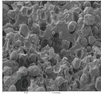
Figure 10. SEM micrograph of tensile fracture surface (51 p.h.r. starch).
