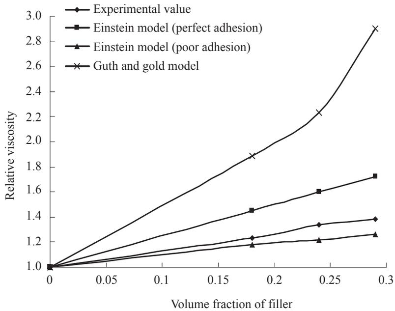
Figure 2. Plot of relative viscosity against volume fraction of starch in the natural rubber compound.
