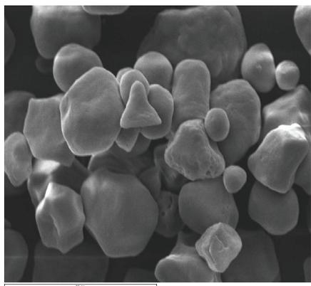
*Figure 3a. SEM micrograph of corn starch.*
