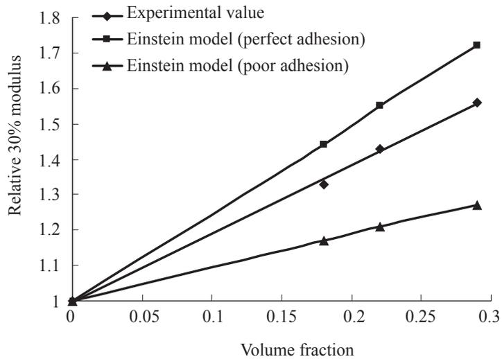
Figure 13. Plot of relative modulus against volume fraction of starch in the natural rubber compound at 30% elongation.
