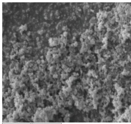
*Figure 3b. SEM micrograph of carbon black (N660).*
