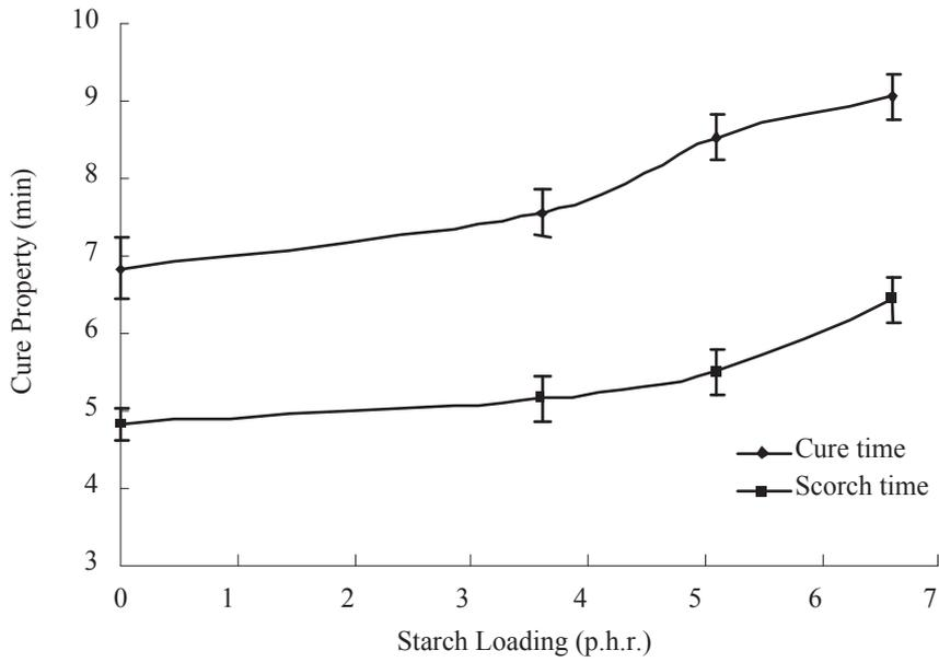
Figure 6. Influence of starch loading on cure properties of the natural rubber compound.
