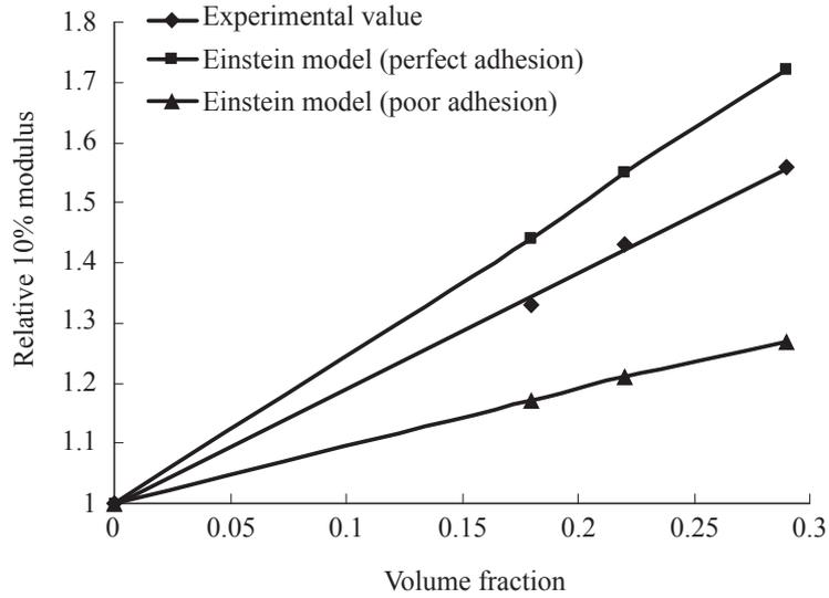
Figure 12. Plot of relative modulus against volume fraction of starch in the natural rubber compound at 10% elongation.
