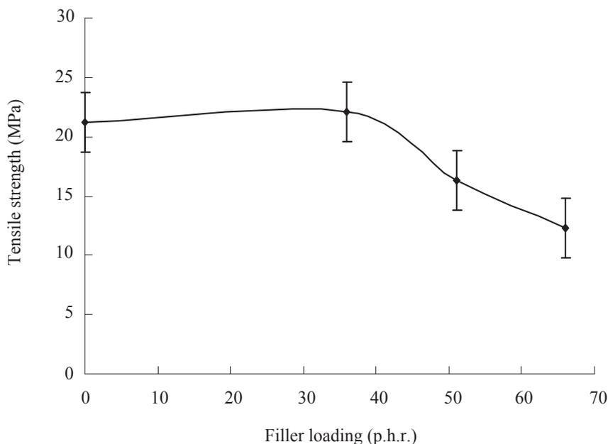
Figure 8. Variation of tensile strength as a function of starch loading in the natural rubber compound.
