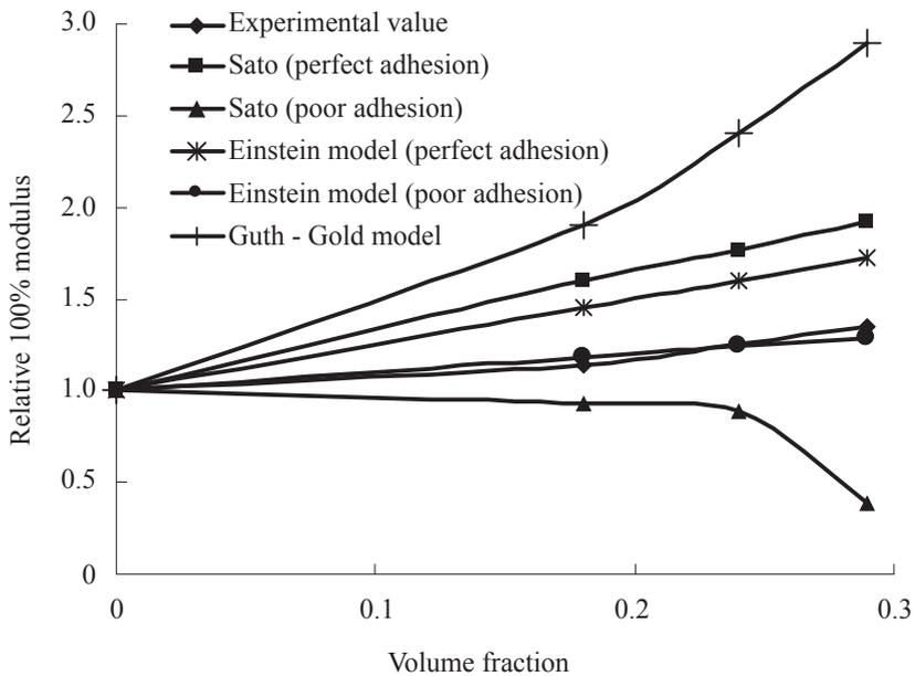
Figure 15. Plot of relative 100% modulus against volume fraction of starch in the natural rubber compound.
