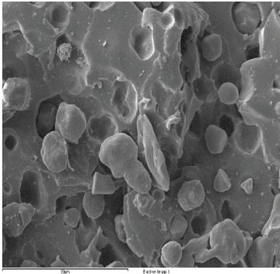
Figure 9. SEM micrograph of tensile fracture surface (36 p.h.r. starch).
