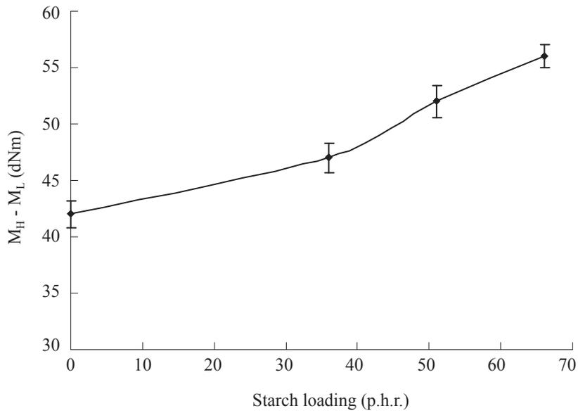
Figure 4. Influence of starch loading on curemeter torque properties of the natural rubber compound.
