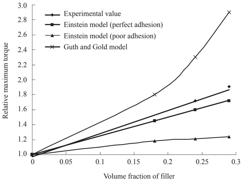
Figure 5. Plot of relative of maximum torque against volume fraction of starch in the natural rubber compound.
