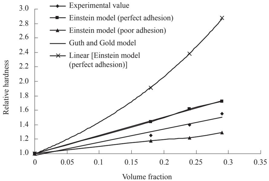
Figure 7. Influence of starch loading on hardness of the natural rubber compound.
