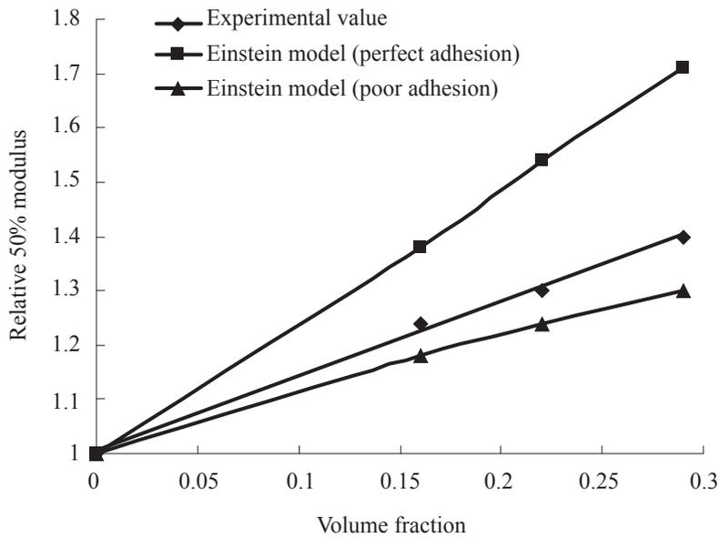
Figure 14. Plot of relative modulus against volume fraction of starch in the natural rubber compound at 50% elongation.
