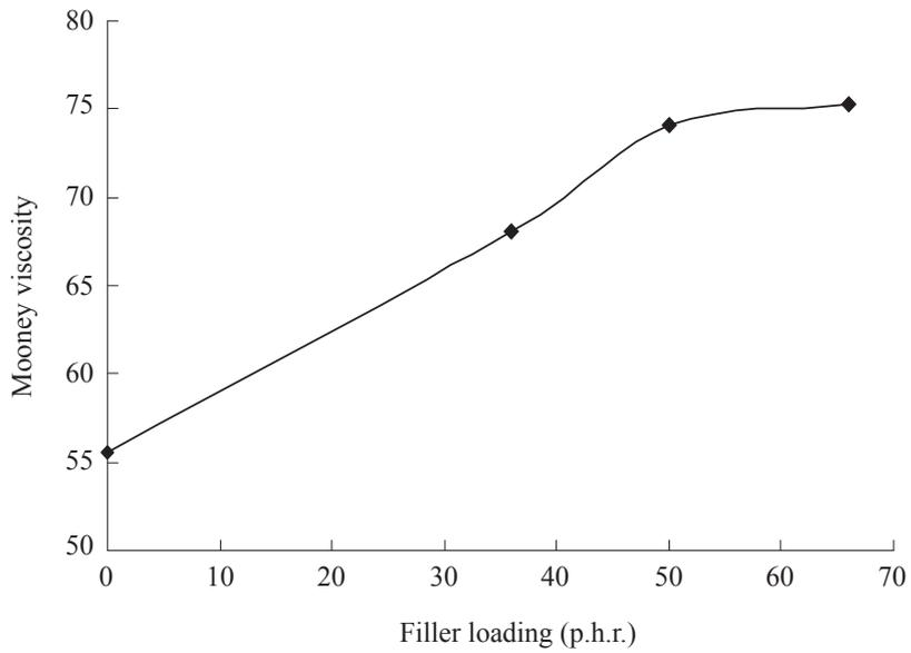
Figure 1. Variation of viscosity with starch loading in the natural rubber compound.
