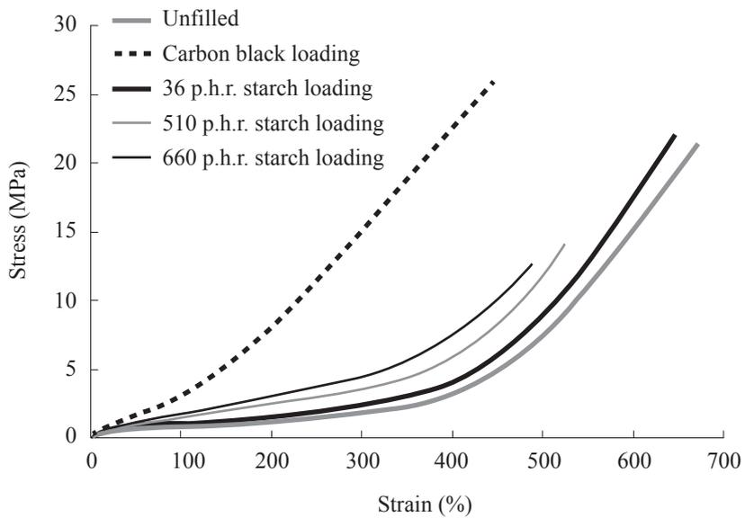
Figure 11. Effect of starch loading and carbon black filler on the tensile stress – strain curve of the natural rubber compound.
