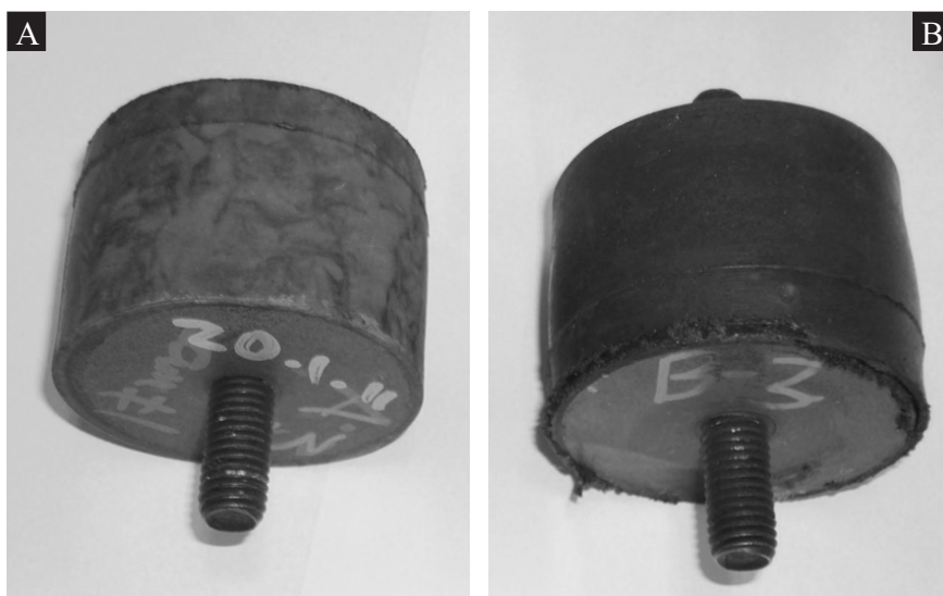
Figure 2. Difference between the surfaces of the bobbins after 60 days in storage at ambient temperature. (A) Compound 1 shows white bloom and (B) Compound 2 shows a clean surface.
