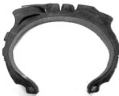
Figure 1. Cross section of a truck tyre that failed by blowout at the thick shoulder region.
