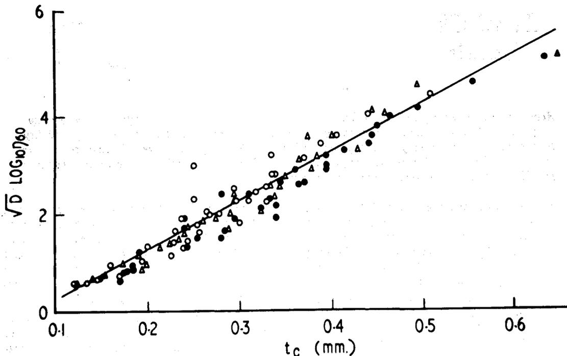
Figure 9. Graph of  $\sqrt{D} \log_{10} \eta_{60}$  and thickness of coagulant dip ( $t_c$ ).
