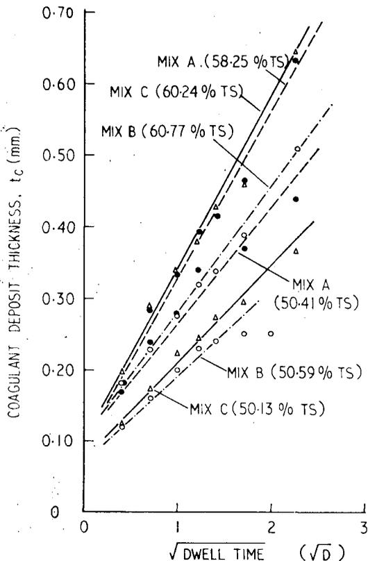
Figure 7. Coagulant deposit thickness and  $\sqrt{D}$  (dwell time).
