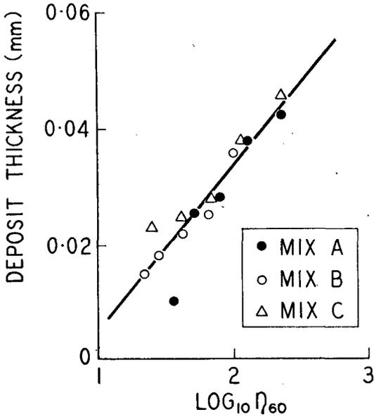
Figure 2. Straight dip deposit thickness and  $\log_{10} \eta_{60}$ .
