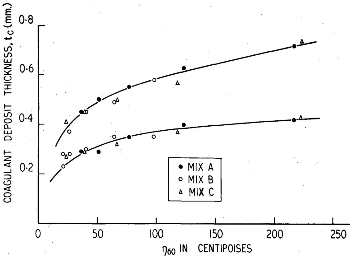
Figure 4. Coagulant deposit thickness and latex viscosity  $\eta_{60}$ .
