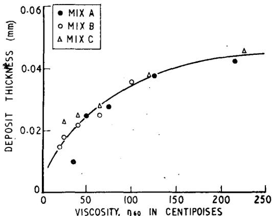
*Figure 1. Straight deposit thickness and latex viscosity  $\eta_{60}$ .*
