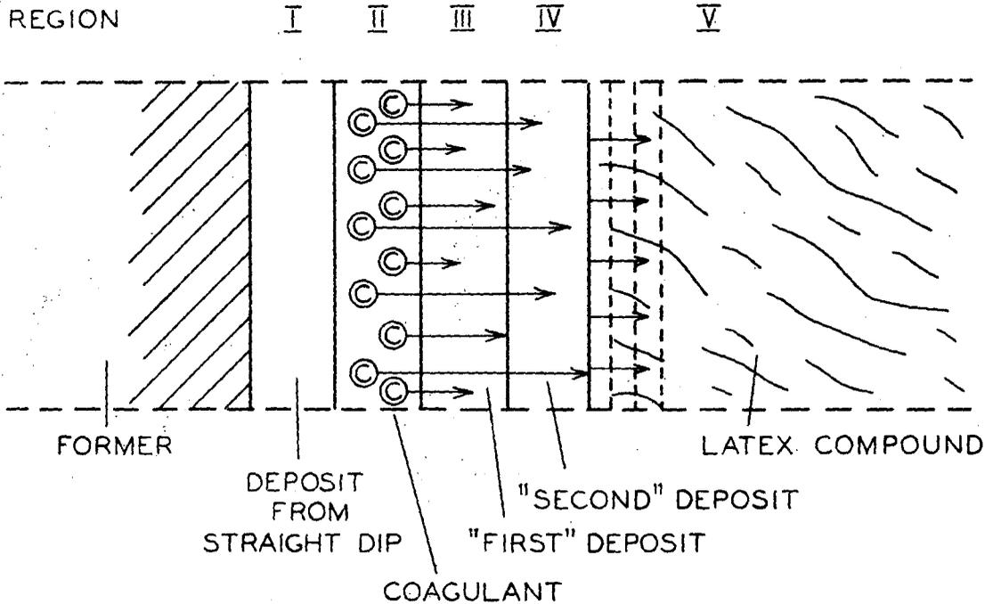
Figure 6. Cross-section of coagulant dipping deposition.
