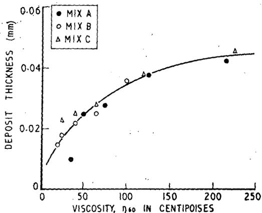
*Figure 1. Straight deposit thickness and latex viscosity  $\eta_{60}$ .*
