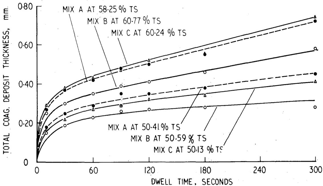
Figure 5. Total coagulant dip deposit and dwell time.
