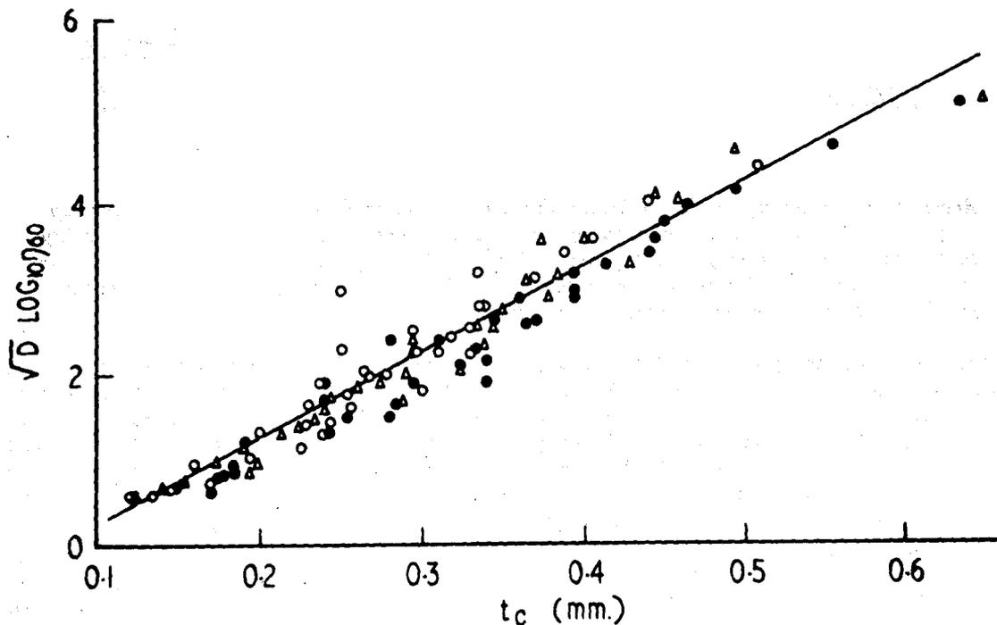
Figure 9. Graph of  $\sqrt{D \cdot \log_{10} \eta_{60}}$  and thickness of coagulant dip ( $t_c$ ).
