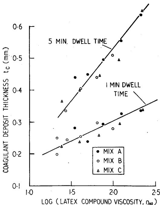
Figure 8. Coagulant deposit thickness and  $\log_{10} \eta_{60}$ .
