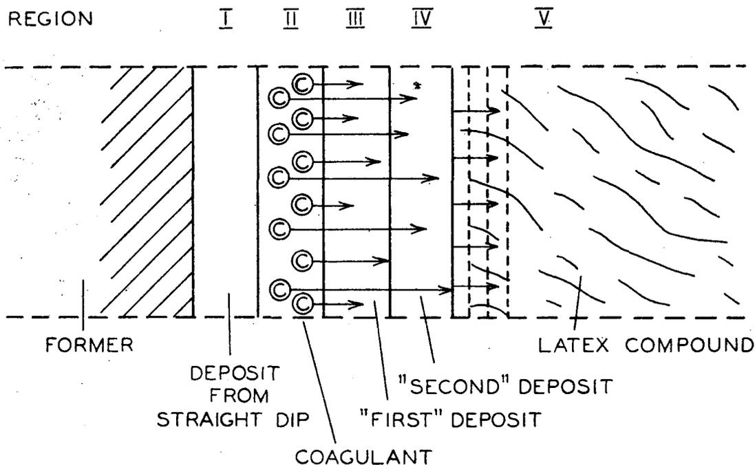
Figure 6. Cross-section of coagulant dipping deposition.
